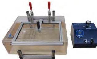
The TME Pressure Bubble Tester provides low pressure and controlled flow to apply to a pouch to meet the requirements of ASTM International F-2096 test method "Standard Test Method for Detecting Gross Leaks in Packaging by Internal Pressurization (Bubble Test)".
