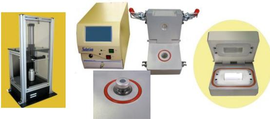
Test systems are available for non-destructive pressure or vacuum testing of sealed bottles containing liquids (vertical fixtures) or solids (vertical or horizontal fixtures), as long as some air space is present inside the bottle. Fixtures can be semi-automated or manual, and the test systems, based around the TME *Solution-C* test instrument, are high resolution, repeatable, and have data storage capability that meets CFR Part 11 guidelines.
