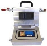
This TME *Solution-C* Chamber Leak Test System is comprised of a pressure decay chamber fixture with a TME *Solution-C* single port pressure decay leak test instrument. The product under test is a foil package containing a vacuum-packed food product. This test fixture is designed with manual toggle clamps as a safety feature.
