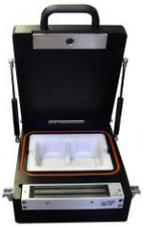
This package test system, consisting of an application-specific fixture and the TME *Solution-C* high-resolution pressure/vacuum leak tester, is configured to perform either vacuum or pressure decay tests at the customer's discretion, but will use vacuum decay for this application. This fixture is designed to perform a vacuum decay test on a two-chamber, thermoformed tray with a welded film cover that contains a medical device. leakage of air ("vacuum decay").
