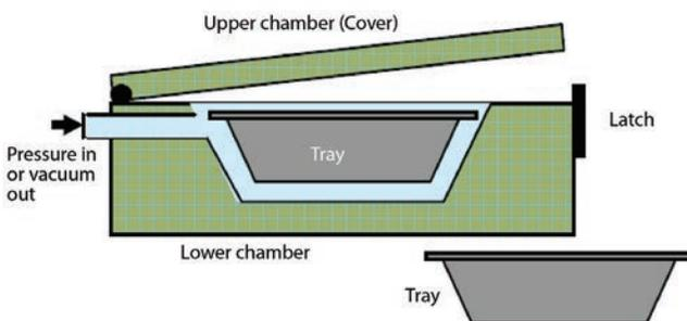
Typical chamber fixture to accommodate pre-formed, filled and lidded trays
