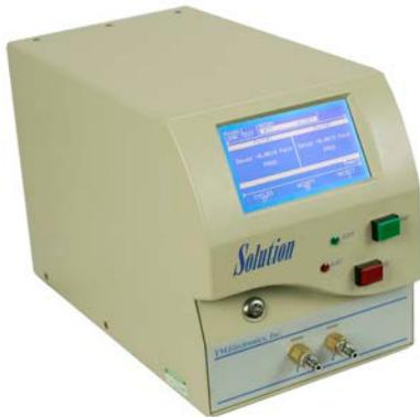
The TME SOLUTION-C test system produces quantitative test results from products that cannot be accessed to pressurize through an access port, as well as sealed, flexible medical, pharmaceutical and food packages. By combining the sensitivity of pressure or vacuum decay leak testing with the simplicity of sealed fixtures, the TME SOLUTION-C system can detect holes as small as 5 microns.
