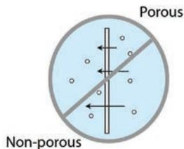
Paper and Tyvek® are not suitable for this type of testing, as they are porous to air movement. Examples of closed products suitable for chamber testing include closed ended extrusions, vials, bottles, and welded housings.
