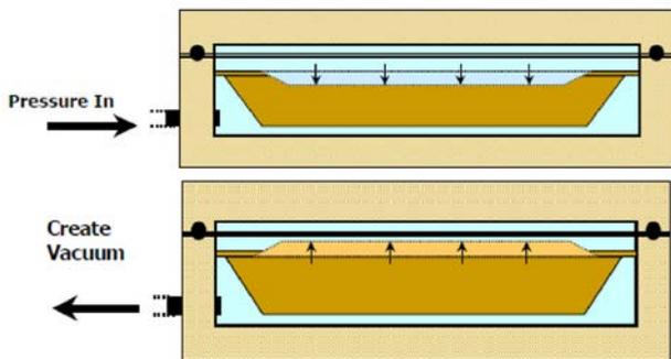
Pressure decay testing is generally the method of choice, because the nature of the pressure decay test allows greater consistency and repeatability in your test results.
