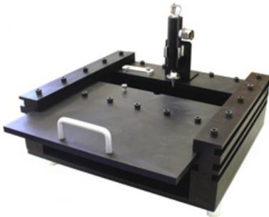
**Restraining plate fixture** - stabilizes expansion during pressure decay testing
