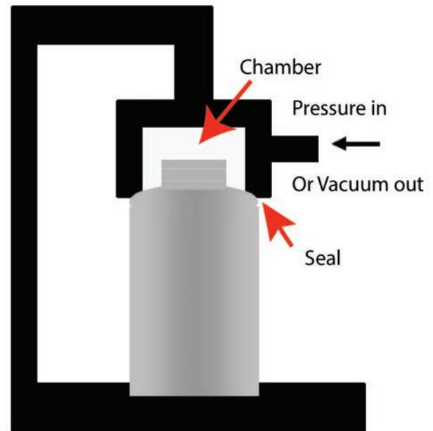
Fixture for non-destructive testing of induction welded bottle seals
