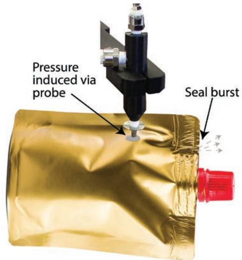
An illustration of seal test
