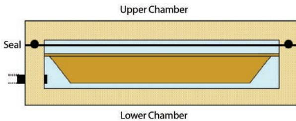
The chamber must be sealed from the atmosphere. This creates the vacant space that will be pressurized or vacated to perform the test. Care must be taken that the seal is strong enough to prevent air leakage when pressurized or vacated. When the test pressure in the chamber space has been stabilized, you will measure leakage by pressure change in vacant chamber space over a predetermined period of time as pressure leaks into (or out of, in case of vacuum test) the test item or package.
