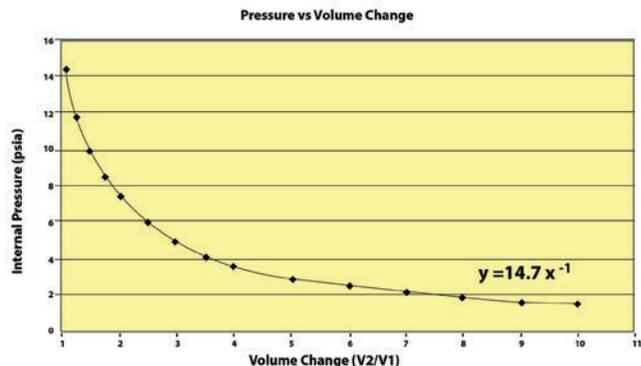
According to this, we see how pressure and volume are related. Therefore, if there is variation in the expansion of test items in a consistent vacuum, then it follows that the volume of the interstitial space, where we are measuring vacuum decay, would vary from test to test. This would make it very difficult to achieve repeatability in test results.
