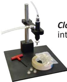
**Closed package test fixture** - for closed package seal strength and leak integrity measurements - includes probe assembly and package access kit
