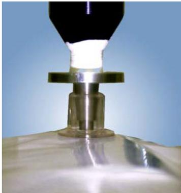
An example of a leak tight path to a package, enabling pressure to be inserted into the package
