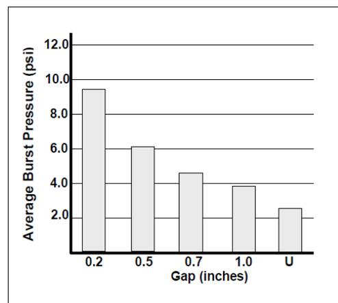
Graph demonstrating average burst pressure to gap width
