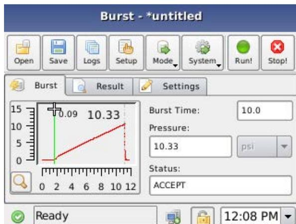
Example of a characteristic burst curve
