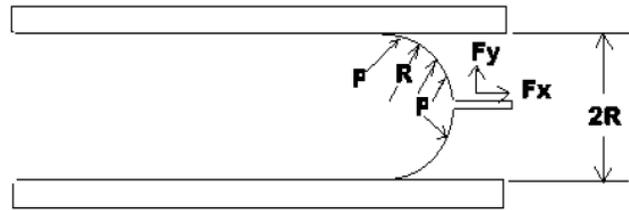
Restraining plate test forces on pouch where  $R$  is the radius,  $P$  is the pressure exerted on the unrestrained edges of the pouch, and  $F_y$  and  $F_x$  are the force vectors on the seal.
