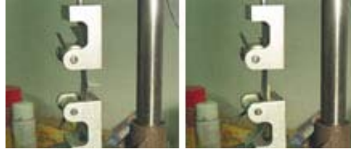
Figure 6. Test sample fixturing using (left) free-tail and (right) supported-tail methods
